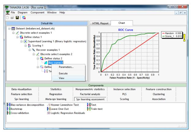
In fact, M2 is not better than M1. The AUC criterion is 81.5%, it was previously 84.5%. The balancing of the learning set by downsizing has no effect on the ability of the classifier to assign higher score to positive instances. M2 is even slightly less efficient because we have reduced the training sample size.
