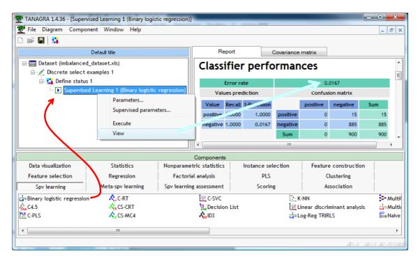
We observe from the confusion matrix that the classifier assigns all the instances to the negative class. The resubstitution error rate seems very small (1.67%). But it is not better than the one of the default classifier. Yet there was no error. The modeling process has run smoothly, we see below the coefficients of the logistic regression.
