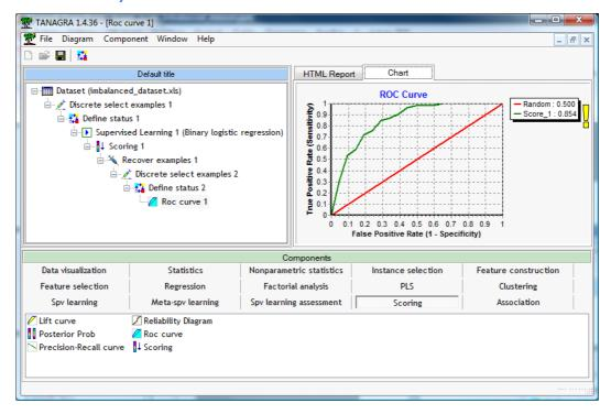
Into the "HTML REPORT", we have the details of calculations. The curve is actually computed on the test set. There were 54 positives among 3000 instances.
