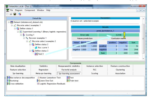
We note above all that the confusion matrix is not suitable to evaluate the performance of classifiers when we deal with imbalanced dataset. The ROC curve shows that we have an efficient model, better than the default classifier. The confusion matrix and the error rate are not able to show it in our very specific context.
